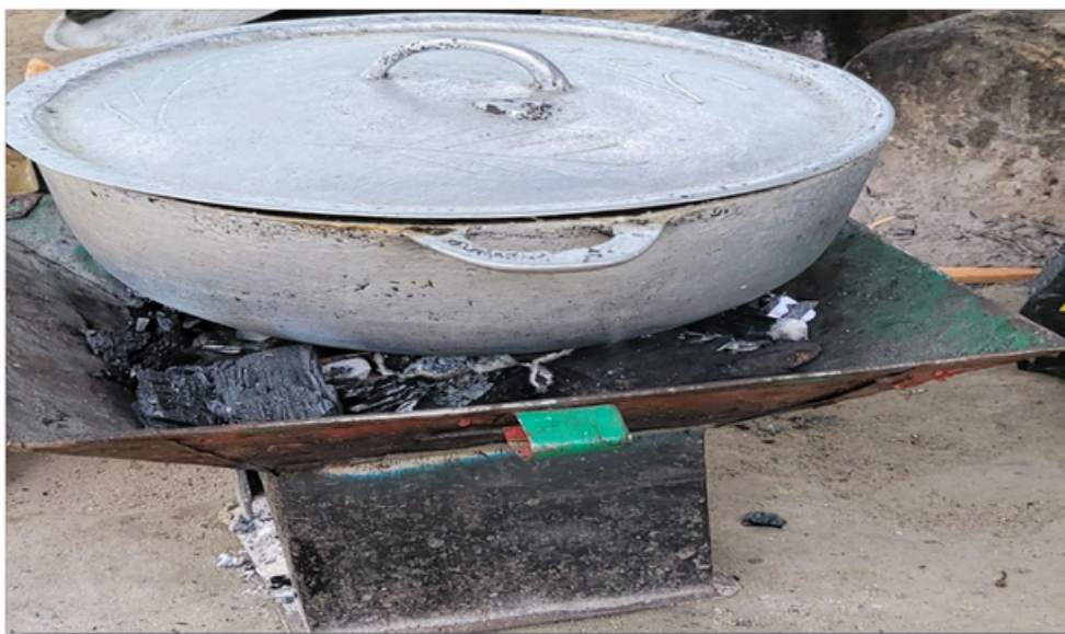
Figure 6 illustrates a locally made charcoal cookstove made out of scrap metals
